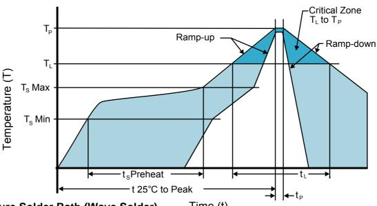
**Low Temperature Solder Bath (Wave Solder)** Time (t)
