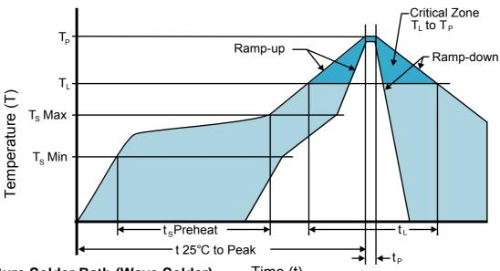
High Temperature Solder Bath (Wave Solder) Time (t)
