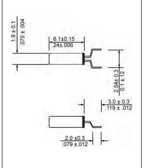
NOTE: Solder by terminals only max 245°C for ten seconds
