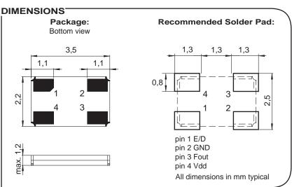
SMT Clock oscillator in ceramic package Fundamental quartz mode frequency
