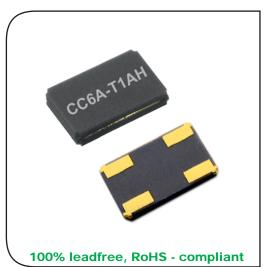
Suitable for Downhole application SMT ceramic package height 0.9 mm Fundamental mode up to 40MHz Extremes temperature ranges High stability and low aging High shock and vibration resistance Hermetically sealed Ultra low MSL Excellent solderability Swiss made quality Customer specification on request
